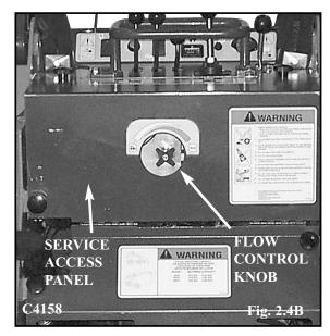
Turning the flow control knob clockwise will divert oil from the loaders drive system to the motor spool auxiliary circuit slowing the loaders travel speed. When fully turned in, approximately 1 gpm (3.8 l/m) of oil will still flow to the loaders drive system. This is the loaders slowest travel speed setting.
