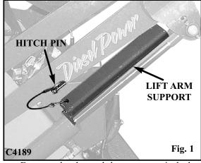
Ensure nylon lanyard does not get pinched or broken. If it does, replace immediately.
