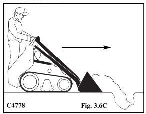
5. Tilt bucket forward as soon as it reaches the edge of the hole and when necessary raise the arms to empty the bucket. (FIg. 3.6D).
