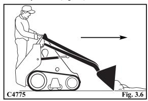
2. To level a filled area, tilt bucket forward and drive machine backwards to drag bucket and spread material (Fig. 3.6A).
