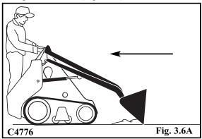
Another method of levelling is to travel forward with bucket down and level, full of material and pushing excess into low areas. Depth is controlled by tilting the bucket slightly up or down. (Fig. 3.6B).
